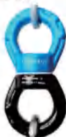
GW-C09 Size:11.1×5.2cm Material: Alu. 6082 Weight: 130g Tension:40KN
