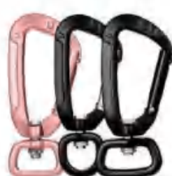
GW-C06 Size:15.5mm, 16mm, 20mm, 25mm Material: Alu. 7075 Weight: 22.4g Tension: 4KN
