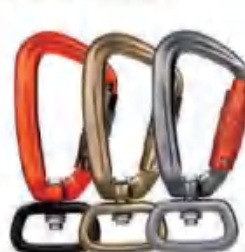
GW-C07 Size:15.5mm, 16mm, 20mm, 25mm Material: Alu.7075 Weight: 25.6g Tension: 4KN
